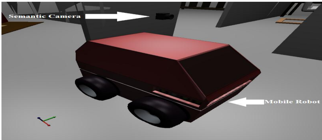
Fig.(3) the camera fixed on the mobile robot.
