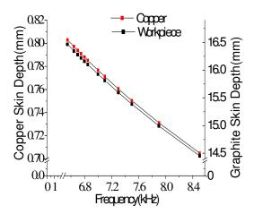
Figure (5). Skin depth at different frequency
