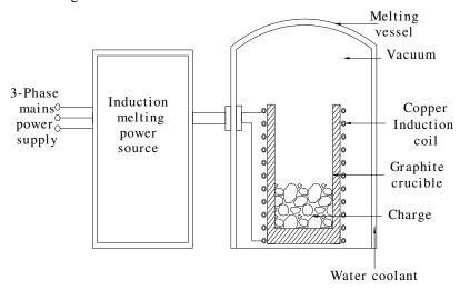
Figure (3). Schematic diagram of Uranium melting
