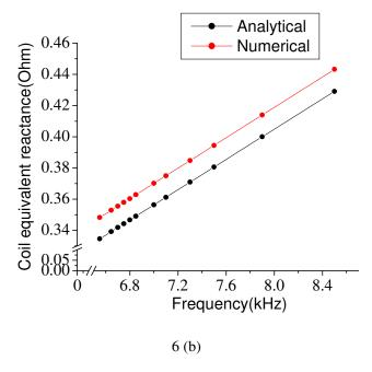
Figure 6(a) coil and workpiece equivalent resistance, 6(b) Coil and workpiece equivalent reactance
