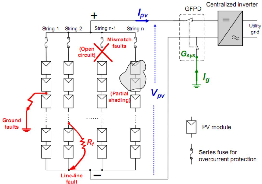
Figure 3. Typical faults in solar PV arrays
