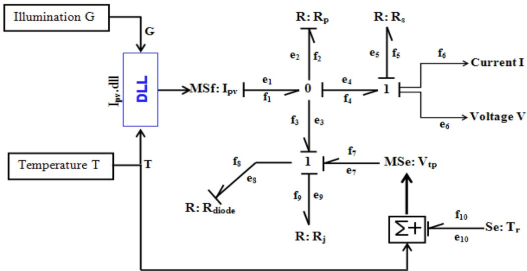
Figure 2. PV Bond graph model with single diode
