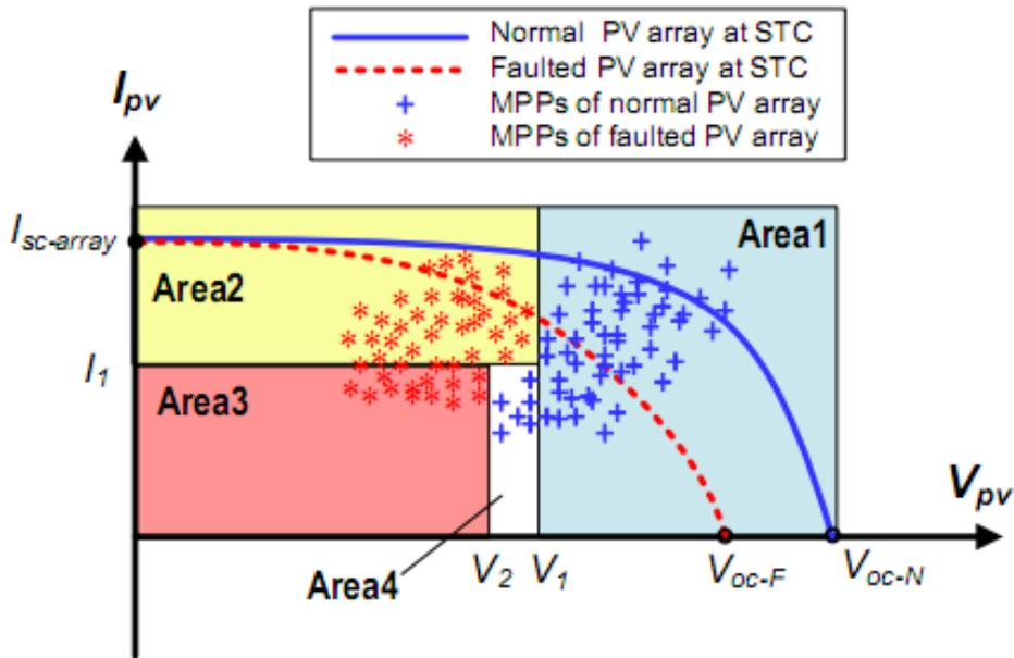
Figure 4. I-V curves of normal and faulted PV arrays
