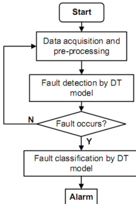
Figure 5. The flowchart of proposed fault detection model
