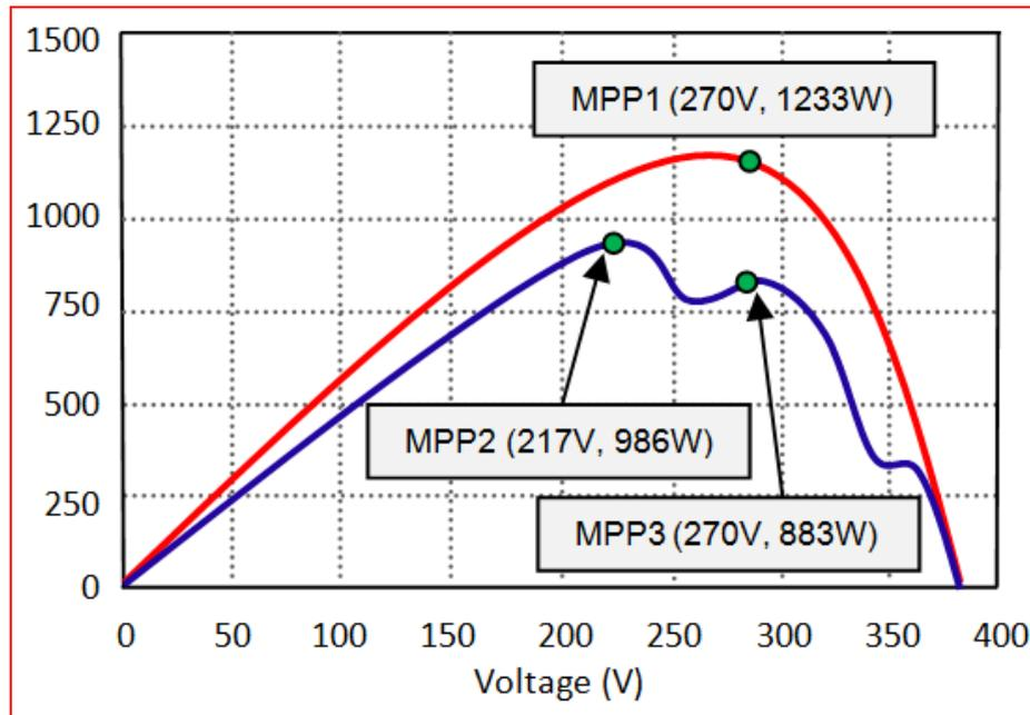
Figure 9. P-V characteristic from offline simulation (case2)
